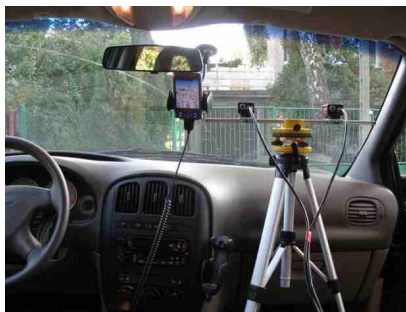
Fig. 6. The experimental road signs recognition system installed in the car
