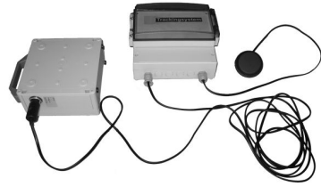
Fig. 2. The implemented prototype of the container tracking unit
